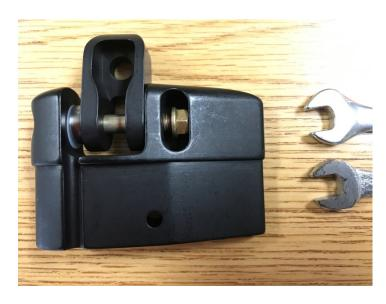
Route the upper VG rope around the inside of the bearing and through the slot in the downtube plug, and re-attach the pulley to the upper VG rope.
