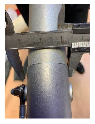
Sprog Bolt is overtightened, compressing the tube out of round
